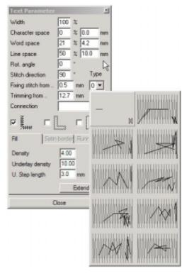
Here the sequence for tack stitch and lock stitch can be edited separately. The tack stitch sequence correlates to position (0,0) at left bottom. The lock stitch sequence correlates to position (6,0) at right bottom.
